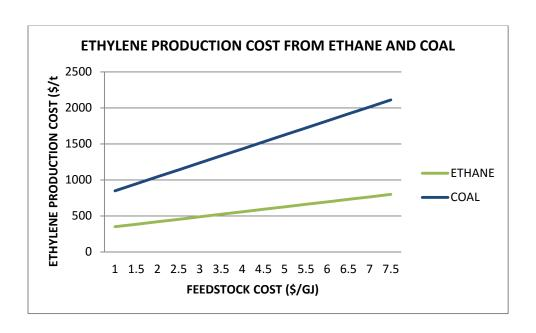
The diagram clearly illustrates the cost advantage of using ethane steam cracking to produce ethylene mainly as a consequence of the lower capital cost (lower intercept on the ordinate axis) and the steeper slope of the line which reflects the lower thermal efficiency of the process - 30% for coal compared to about 77% for ethane cracking.
